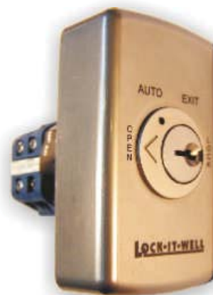
The Example shown is for a Auto Series Lockwood 6-pin inline mullion mount, with key removal in 4 positions Multi-Voltage switch.
